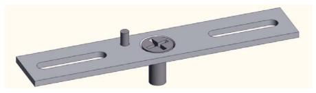
Step 2: Pull Aircraft suspension cable through the slot of 2 piece coupler until its end and fasten top coupler cover.
