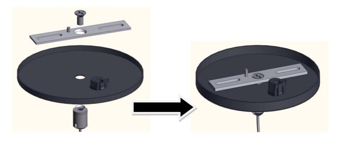
Step 4: Installing cable (A) in Gripper (C)
