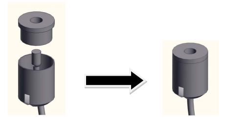
Step 3: Fasten Crossbar (step 1) with canopy and 2 piece slotted coupler
