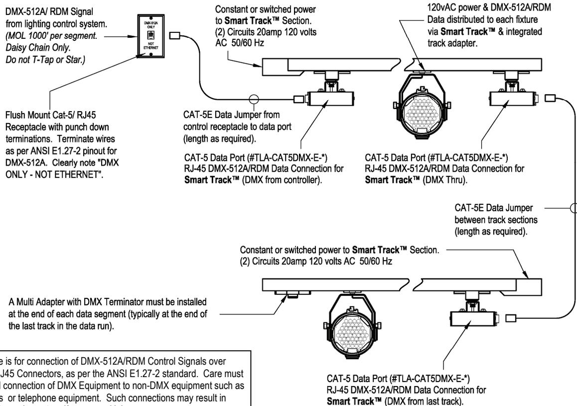
**Note:** This device is for connection of DMX-512A/RDM Control Signals over Cat5 wiring via RJ45 Connectors, as per the ANSI E1.27-2 standard. Care must be taken to avoid connection of DMX Equipment to non-DMX equipment such as Ethernet switches or telephone equipment. Such connections may result in serious damage to equipment and/or personal injury.
