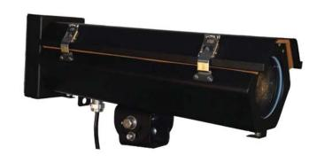
The lid is secured to the body with four side-mounted link-lock latches that provide a water tight seal. Padlocks of appropriate size can be added for security. The proprietary highly polished reflector is engineered for use with T6 G12 CDM/CMH lamps for maximum output. The lens focus adjustment is via Teflon guides throughout the focus range. Focus is secured by way of brass thumb screws.
