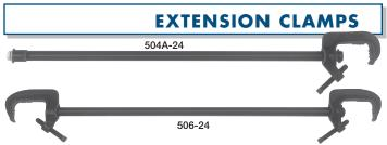
504A extension clamps are for extending the mounting position of luminaires from pipe battens. They are provided with a 510 pipe clamp on one end, and a 1/2"- 13 attachment bolt with washers on the other. 506 extension clamps are provided with a 510 pipe clamp on each end for hanging one pipe from another. All items are finished in baked black enamel.
