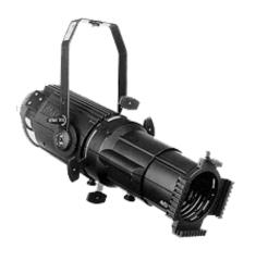
The Altman Shakespeare Ellipsoidal Spotlight is a high performance fixture that stands out against the competition. Features include die cast construction, a high-efficiency "cool beam" Dichroic glass reflector, rotating shutter & gate assembly, and superior projection of metal or glass patterns.
