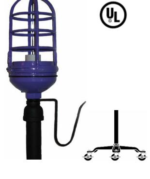
The Behind the Scenes Ghostlight comes with the protective basket and base assembly finished in Behind the Scenes Purple. The stand and locking three-wheeled base are finished in black enamel. The unit is furnished with a 15' 12/3 SJ cable with a parallel blade and ground connector; cable hook; and a medium screw-base socket. The unit is UL-Listed as a Portable Luminaire, Issue BK 09976 and is rated for a 100-Watt maximum Type A lamp.
