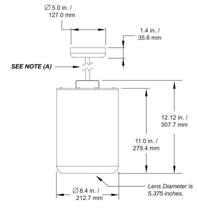
**NOTE (A) Specify Length of:** Stem: 6 in. / 152.4 mm to 72 in. / 1.8 m Aircraft Cable: Up to 20 ft. / 6.1 m
