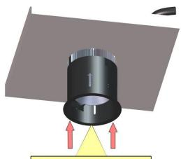
Cut a 6" hole in the Ceiling. Insert the Fixture into the Ceiling hole.
