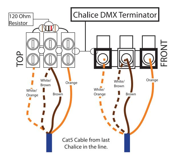
DMX termination for Chalice should be installed on the DMX Cat5 cable bare end on the last fixture in the communication line.
