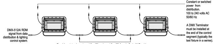
Feed thru data via on-board 2m (6') male and 2m (6') female 5-pin XLR cables. A 12' cable run between fixtures can be obtained without requiring additional DMX-512A data cables
