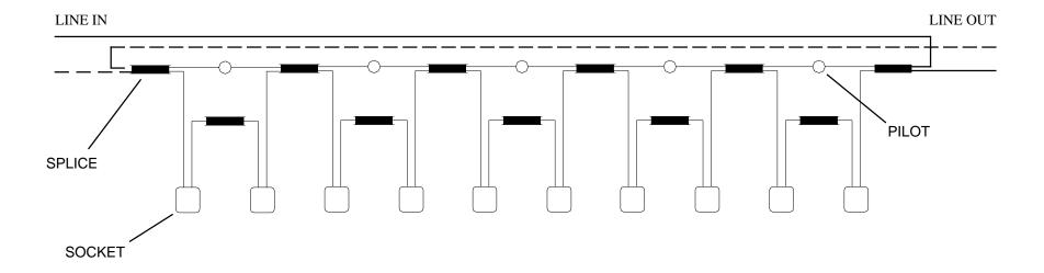
NOTE: This diagram represents a single circuit. A ZS-1 would have 1 circuit, a ZS-2, -3, -4 would have 2, 3, and 4 circuits respectively.
