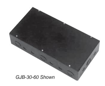
The Gridiron Junction Box is a surface mount wiring device usually attached to the grid. It is used to connect the wires within conduit to the multi-conductor flexible cable which feeds strip lighting devices or connector strips. These boxes may be located anyplace where wire connections are required, and are available in many sizes.
