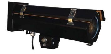
The lid is secured to the body with four side-mounted link–lock latches that provide a water tight seal. Padlocks of appropriate size can be added for security. The proprietary highly polished reflector is engineered for use with T6 G12 CDM/CMH lamps for maximum output. The lens focus adjustment is via Teflon guides throughout the focus range. Focus is secured by way of brass thumb screws.
