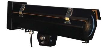
The lid is secured to the body with four side-mounted link–lock latches that provide a water tight seal. Padlocks of appropriate size can be added for security. The proprietary highly polished reflector is engineered for use with T6 G12 CDM/CMH lamps for maximum output. The lens focus adjustment is via Teflon guides throughout the focus range. Focus is secured by way of brass thumb screws.
