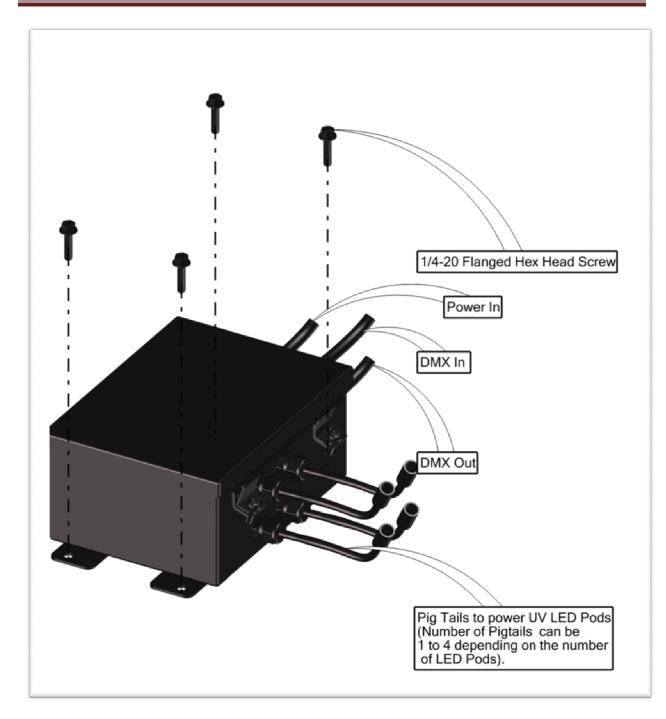
Mount the Control Box in the desired location using suitable hardware. ¼-20 screws are recommended for mounting the Control Box.
