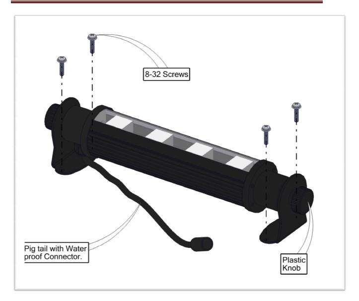
Mount the pods in the desired location using suitable hardware. 8-32 screws are recommended for installing the Pods.
