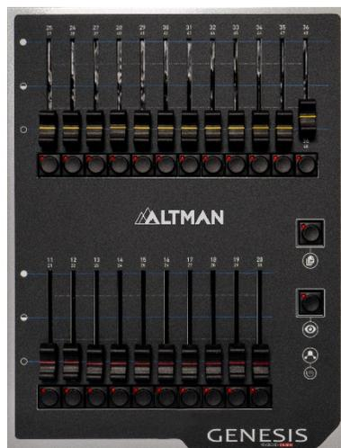
Up to 2 wings can be connected to a Genesis console.
