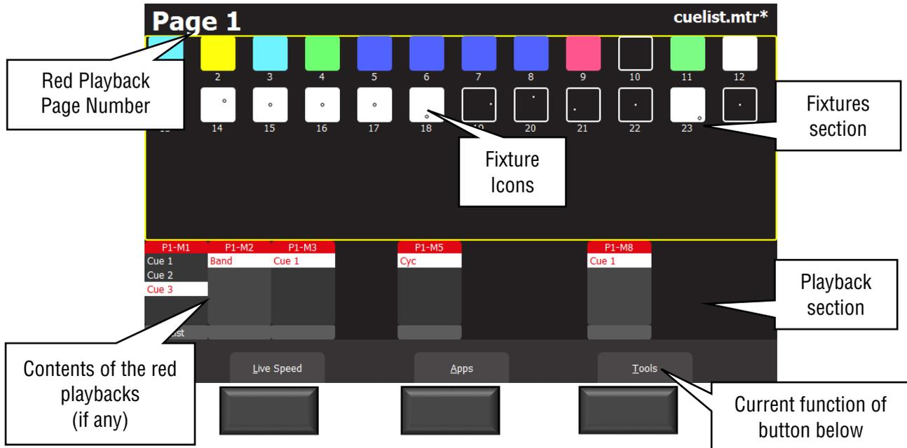
The 3 buttons below the touch screen have different functions for different screens. Their current function (if any) is shown on the screen above each button. Either tap the button or touch the virtual button on the screen to operate them.
