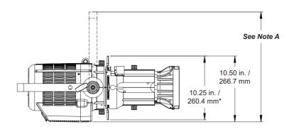
\*Dimensions shown are with shutter blades fully retracted (pushed in).
