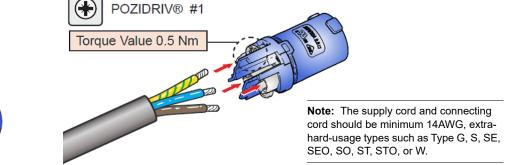
Figure 5: PowerCON (Blue AC Input) Connector Wiring
