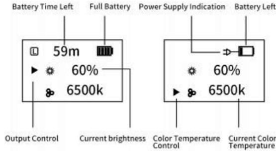
Power Supply indication: the icon will display when power is connected.
