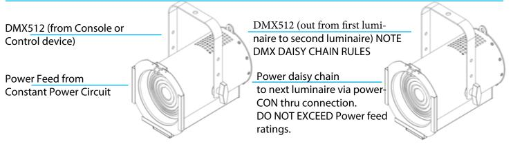
**SPECIAL NOTE:** PEGASUS must be set to DMX CONTROL (switch on the back of the luminare) to be controlled via a DMX 512 system. Please select the Luminaire dim curve for local voltage to either 115VAC or 230VAC. If switching between MAINS CONTROL and DMX CONTROL. Please remove power from Luminiaire and **wait 10 Seconds** before switching the luminaire to DMX CONTROL.
