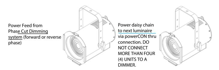
**SPECIAL NOTE:** PEGASUS must be set to MAINS CONTROL (switch on the back of the luminare) to be controlled via a phase cut dimming system. Please select the dimming system dim curve for local voltage to either 115VAC or 220VAC If switching between DMX CONTROL and MAINS CONTROL. Please remove power from Luminiare and **Wait 10 Seconds** before switching the luminaire to MAINS CONTROL.
