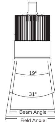
Note: To determine the center beam illumination in Foot candles at any distance, divide Candela by the distance squared.
